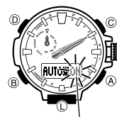
Auto light switch on indicator
