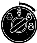
Engine "ON" Position (Normal Operating)
