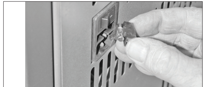
Figure 20b: Main power switch
