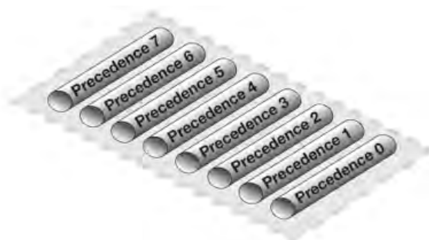
Figure 10.2. The Eight Pipe Precedences.
