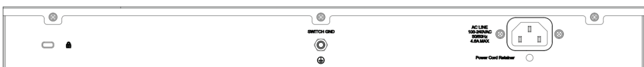
Figure 2-12– DGS-1100-26MPV2 Rear Panel
