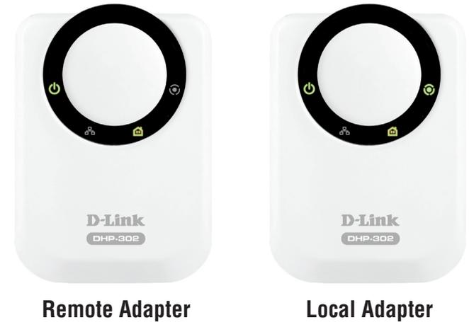
**Note:** When adding more adapters, repeat steps 1 to 3. At the end of this process, only the local adapter should have the AP LED lit.
