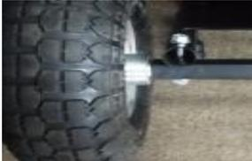
6. Slide 1in. Washer onto each end of the Axle.
