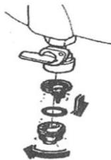
*Fuel Filter Element Removal*
