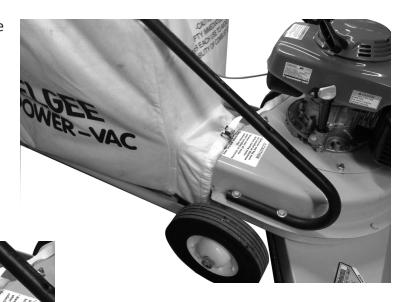
**2.** Cinch the *Filter Bag's* built-in strap to secure its neck.
