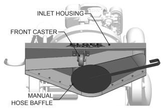
**2C. ONBOARD HOSE BAFFLE:** If your machine is equipped with the optional *Onboard Hose Baffle*, simply press down on the *Baffle Control Handle* to release the locking pin and rotate it clockwise as far as it will go. Note: Pull the machine backwards a few inches before turning the *Baffle Control Handle* in order to ensure there will be no interference with the *Front Caster*.
