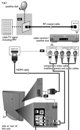
You can also connect this unit to the cable receiver or satellite box other than the HDMI or the component video output jacks because they might have different output jacks.
