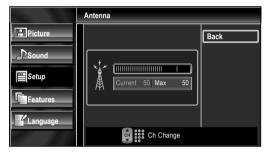
If the channel is set to analog (cable) channel or external input, you cannot confirm the antenna condition.
