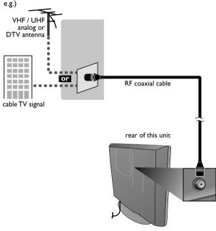
Once connections are completed, turn on the unit and begin initial setup. Channel scanning is necessary for the unit to memorize all available channels in your area.
