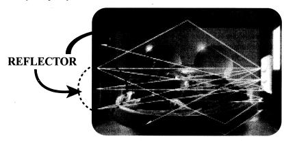
What is the Omni Wave Cooking System™? The Omni Wave Cooking System™ concentrates the waves equally on all areas of the food item. The dual wave system distributes waves evenly into the cavity from two points, one above the item and one below.
