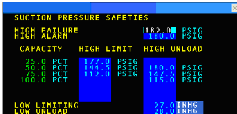
High Suction Pressure Setpoints Screen
