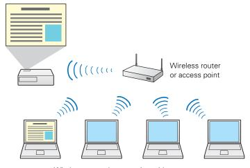
Wireless network connection with interactivity using the built-in toolbar
