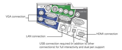
If you connect VGA cables to both the Computer1 and Computer2 ports, make sure you label the cables. The teacher or other user needs to know which port is being used so that the correct source for full interactivity can be selected in the Easy Interactive Function menu screen.
