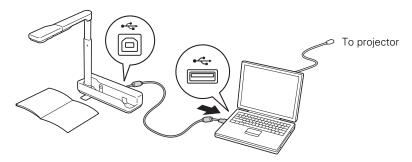
Although you can connect the EPSON DC-06 directly to the projector's USB-A port using a USB cable, this will provide only limited interactivity (using the built-in interactive toolbar).
