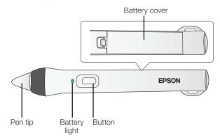
To turn on the pen, tap the pen tip or press the button on the side of the pen. The green light comes on briefly. If the battery is low, the light flashes.  Hold the pen perpendicular to the board, as shown below.
