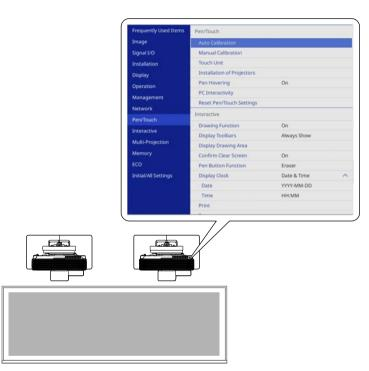
Follow the on-screen instructions to perform auto calibration. If the auto calibration fails, perform **Pen/Touch** > **Manual Calibration**.
