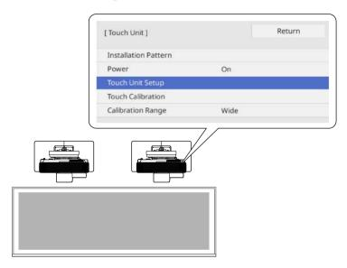
Follow the on-screen instructions to perform touch unit auto adjustment. See your projector's *Installation Guide* for details on the auto adjustment.
