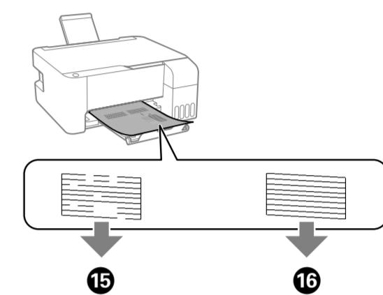
**15** Run the print head cleaning. Print head cleaning uses some ink from all ink tanks.
