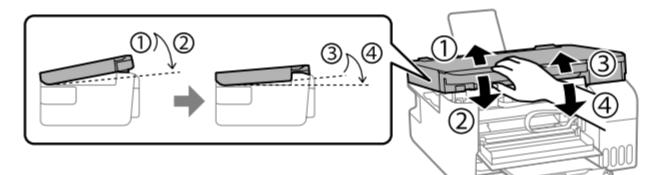
The unit must be closed completely before it can be opened again.
