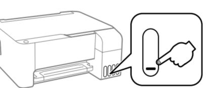
To confirm the actual ink remaining, visually check the ink levels in all of the printer's tanks. Prolonged use of the printer when the ink level is below the lower line could damage the printer.
