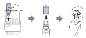
**Note:** Do not leave the ink bottle inserted; otherwise the bottle may be damaged or ink may leak.
