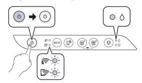
10 Press and hold the ⊕ stop button for 5 seconds until the ⊕ power light starts to flash and ink charging begins. Ink charging takes about 11 minutes.
