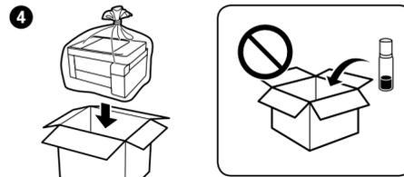
☐ Be sure to keep the ink bottle upright when tightening the cap. Place the printer and the bottle in a plastic bag separately and keep the printer level as you store and transport it. Otherwise ink may leak.
