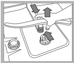
The lower sprayer arm can be removed by pressing on the side tabs and pulling it upwards.
