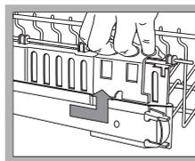
If the rack is fitted with **Dual Space** handles<sup>\*</sup> (*see figure*), pull out the upper rack until it reaches its stop point, grip the handles at the sides of the rack and move it upwards or downwards, then slowly let it fall back into place.
