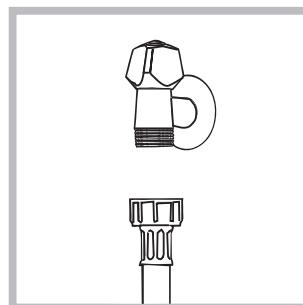
1. Connect the supply pipe by screwing it to a cold water tab using a 3/4 gas threaded connection (see figure).
