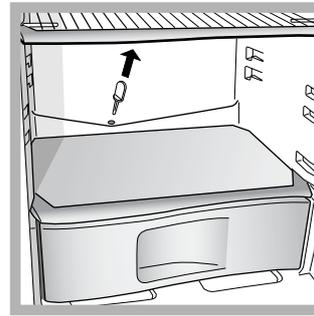
The refrigerator has an automatic defrosting function: water is ducted to the back of the appliance by a special discharge outlet (*see diagram*) where the heat produced by the compressor causes it to evaporate. It is necessary to clean the discharge
