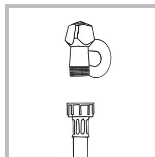
1. Connect the supply pipe by screwing it to a cold water tab using a  $\frac{3}{4}$  gas threaded connection (see figure).
