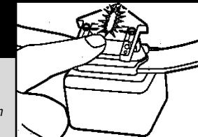
Place test light across skin contacts. Press the "C" button on transmitter, test light will illuminate to show stimulation.
