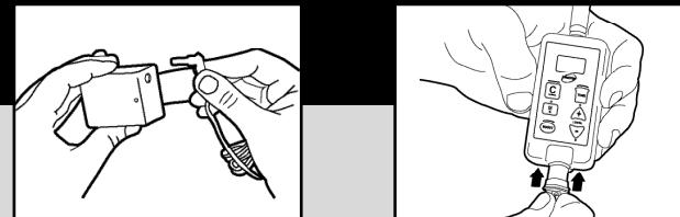
**COLLAR RECEIVER:** Charge the collar 12-14 hours. Be sure to cover the charge jack with the gray plug when done.
