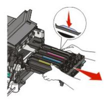
**8** Remove the used developer unit.
