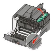
3 Remove the toner cartridges by lifting the handles, and then gently pulling away from the imaging kit.
