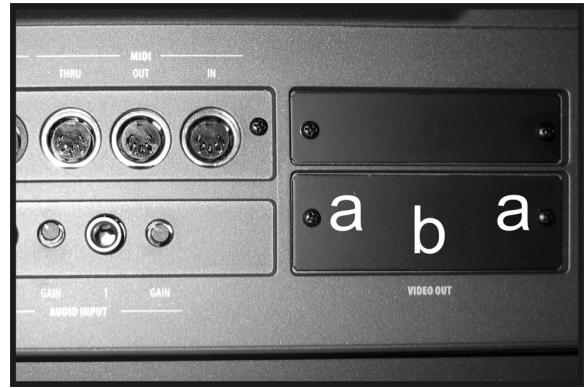
2. Fully remove the cover (b) by unfastening the ground cable (c). Be very careful not to let the ground cable (c) and the attached power cable (d) fall inside the instrument.
