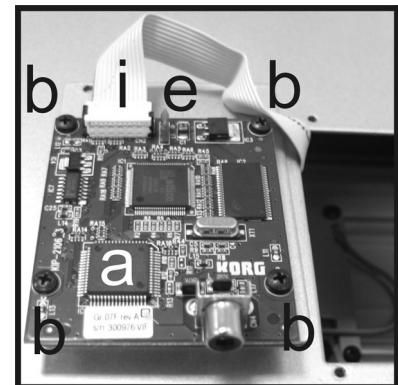
5. Replace the cover (e) to the original position, being very careful to make the protruding side of the circuit board (a) slide in before any other side.
