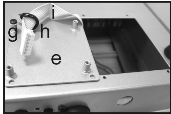
4. Attach the cover (e) to the circuit board (a) by using the four previously removed screws (b). Connect the power cable (i) to the circuit board (a), as shown in the illustration.
