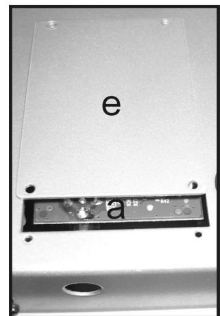
6. Slide the cover (e) up to the original position. The video connector protruding from the circuit board (a) will pass through the corresponding hole on the back of the instrument. Attach the cover (e) to the bottom of the instrument by using the four previously removed screws (d).
