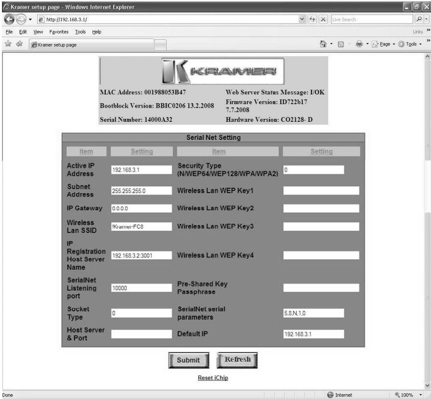
Figure 5: Serial Net Configuration Screen of the FC-8
