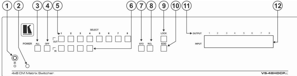
Figure 1: VS-48HDCPxL 4x8 DVI Matrix Switcher Front Panel
