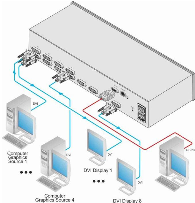
Figure 3: Connecting the VS-48HDCPxI 4x8 DVI Matrix Switcher
