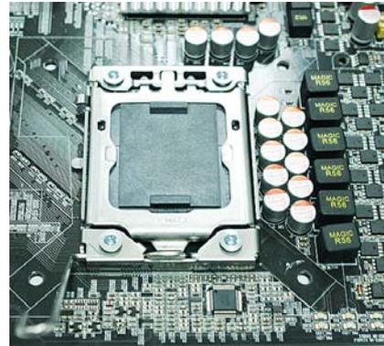
2. Press down the level and move it to the left side to make sure it is freed from the hook and then open it upwards about 135 degree.
