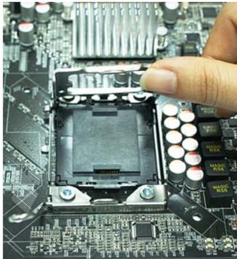
3. Pick up the lode plate upwards about 100 degree to make sure it is moved upwards.
