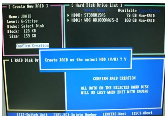
Then press Enter to enter the Confirm Creation item, then dialogue box would show Create RAID on the select HDD(Y/N)?Y. Type Y, and press Enter, the following window would show up to confirm the success in creating RAID mode.
