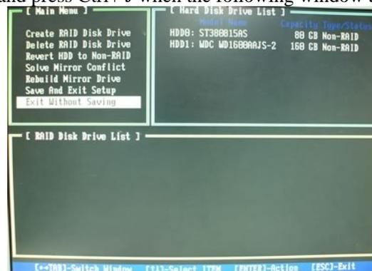
The name disks you would like to set RAID function should appear under the Hard Disk Driver List
