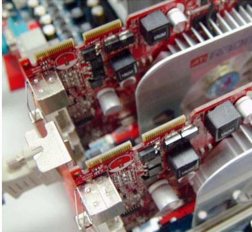
1. Install your CrossFire Tech Supported VGA Cards in the PCI-E x16 slots.
