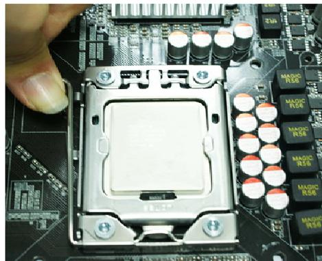
7. Press down the load level and move it rightwards make sure it is locked under the notch.
