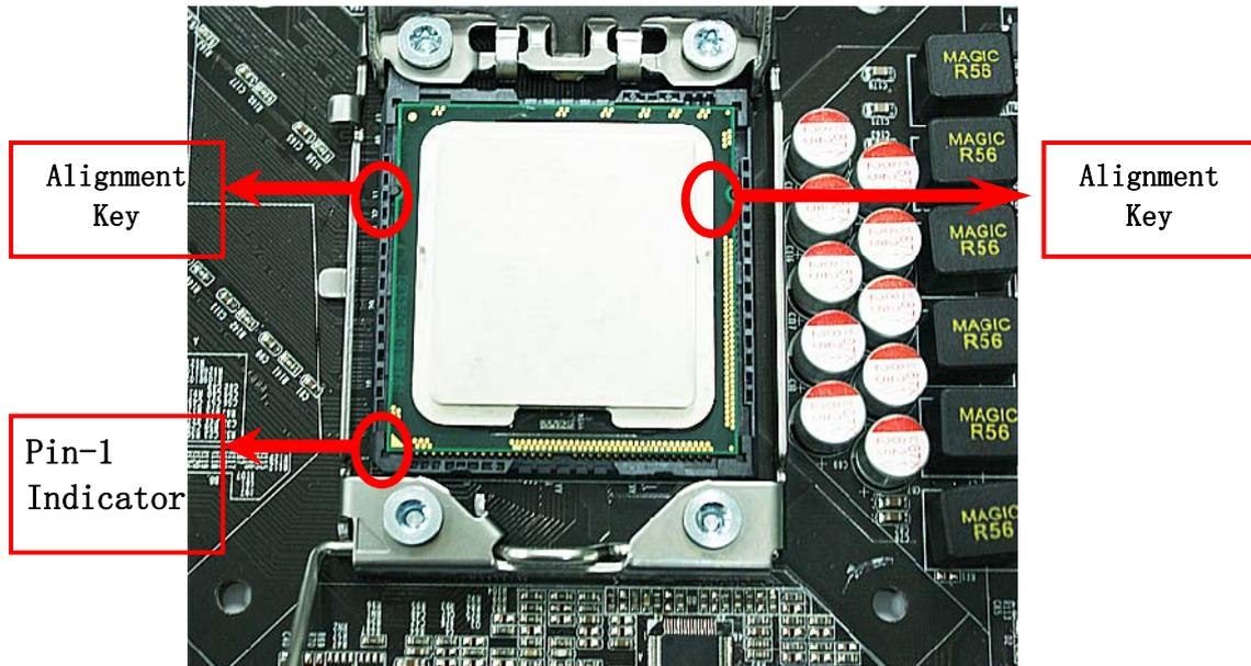
5. Make sure that golden finger is on the left-down side as shown and match the two alignment keys on the CPU with two points of the socket. CPU can only be correctly installed with this direction. Incorrect installation might cause damage to CPU .
