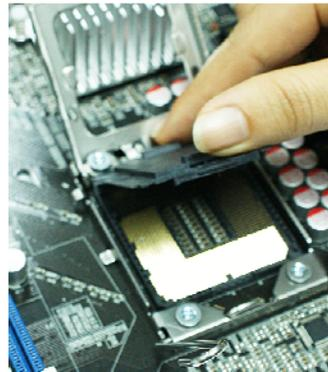
4. Remove the plastic protective cap from the socket. ( Put it to the original place if CPU is not installed . Do not touch the metal contact point of the CPU socket).
