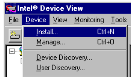
Figure 5. Start the Device Install Wizard. Select Install from the Device menu to start the Wizard.
