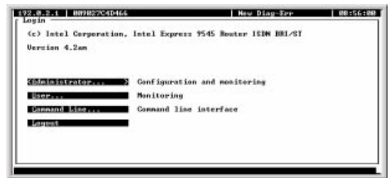
Figure 12. Local Management Login Screen. Use the ↑ ↓ keys on your keyboard to select an option and press ↵ , or type the underlined letter of the option.
