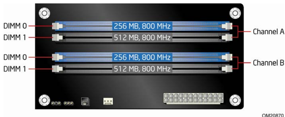
Figure 15. Dual Channel Memory Configuration with Four DIMMs
