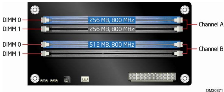
Figure 16. Dual Channel Memory Configuration with Three DIMMs
