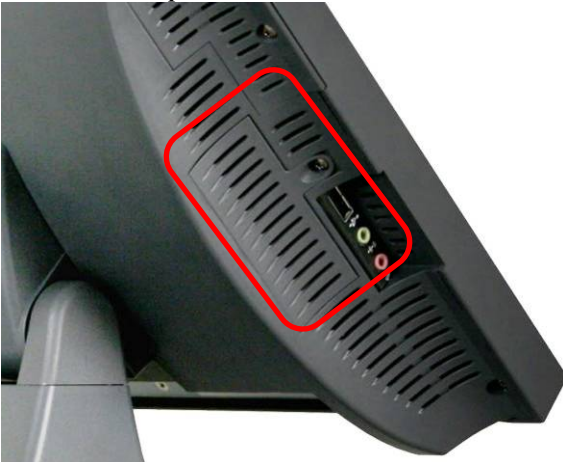
HDD access panel
