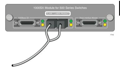
2 Plug the other end of the cable into a device and check the LEDs on the 1000Base Module to verify the link. For information on the LEDs, see Chapter 2.
