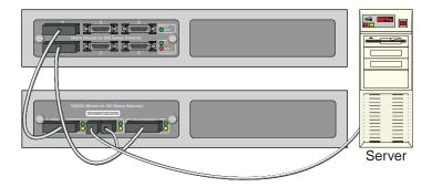
6 Check the LEDs on the 1000Base Module to verify the links. For more information on LEDs, see Chapter 2.
