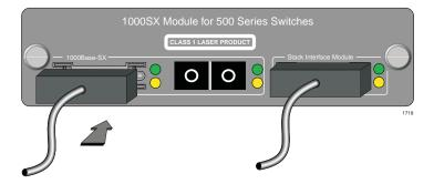
6 Plug the other end of the Stacking Cable into an empty port on the Matrix Module located on the same side of the switch (both modules in Slot A), and secure it using the latches on the connector.
