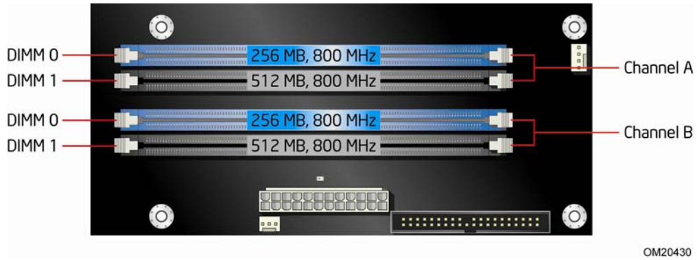
Figure 18. Dual Channel Memory Configuration with Four DIMMs
