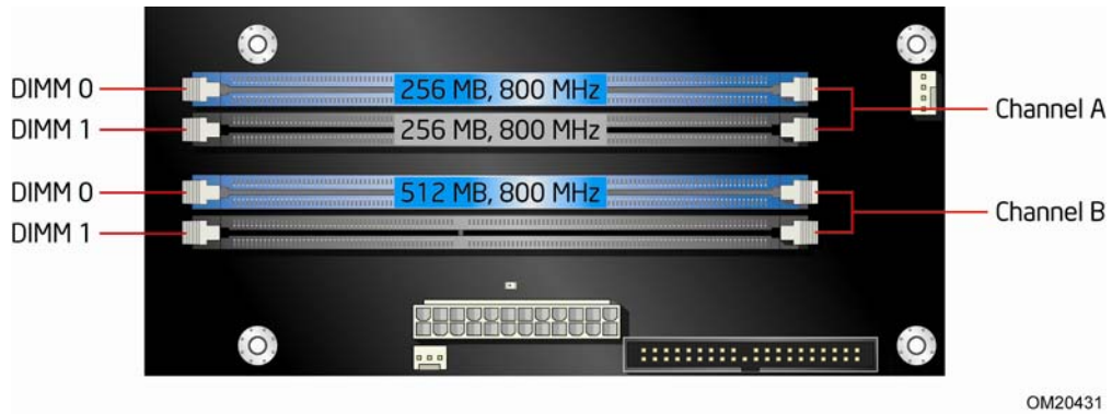
Figure 19. Dual Channel Memory Configuration with Three DIMMs
