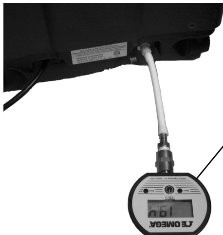
FIGURE 23.2 4 Way Valve Function Test
