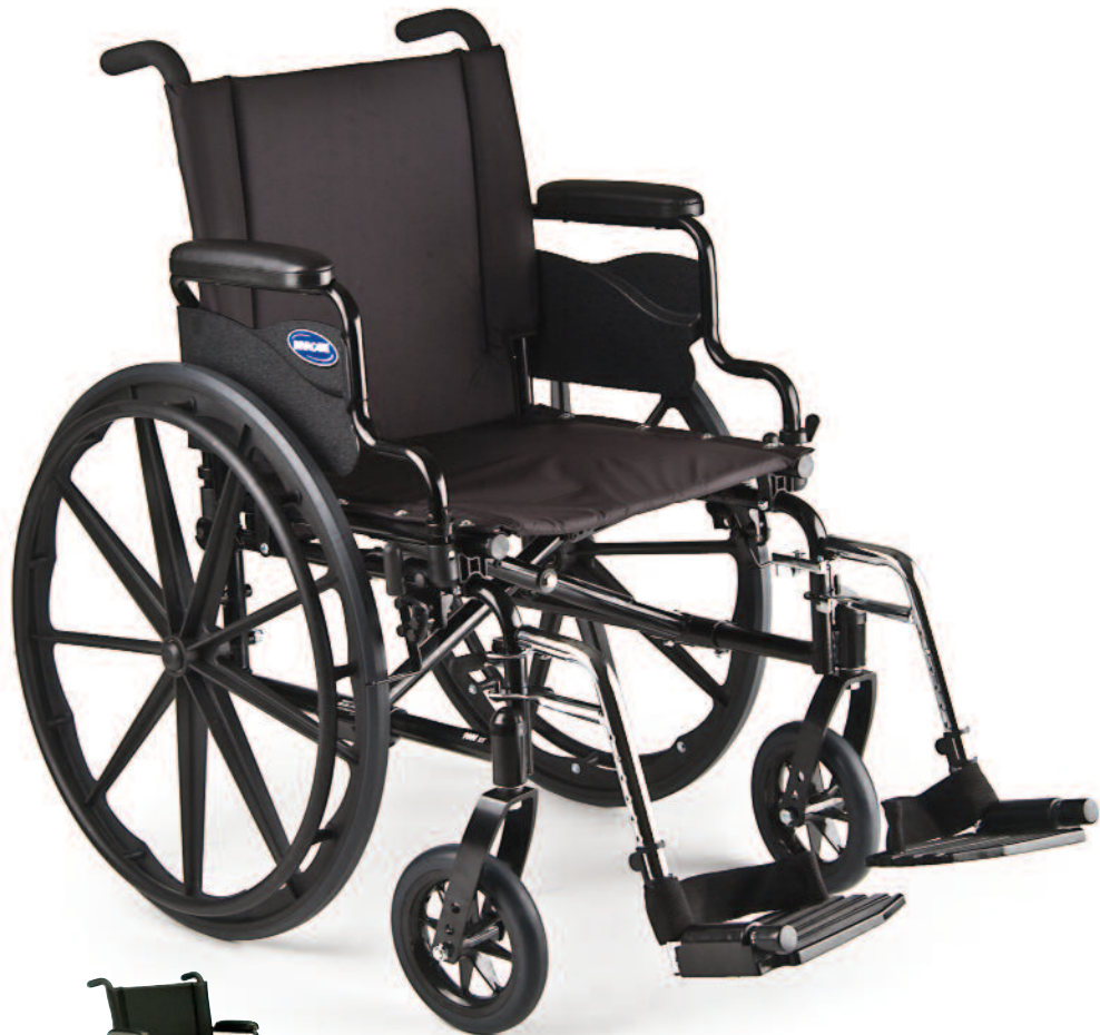
9000 XT wheelchair with offset axle and adjustable angle caster will allow additional seat-to-floor heights and increase seating and positioning capabilities. Offset axle offers center-of-gravity adjustment which increases maneuverability and stability.
