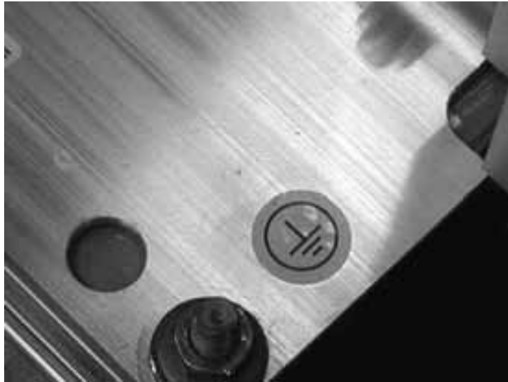
Figure 3-3: Grounding Terminal on Mounting Plate
