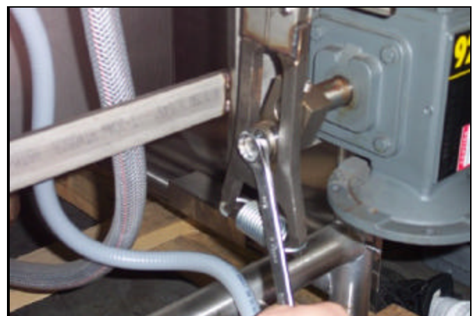
Removing the drive hub bolt.
