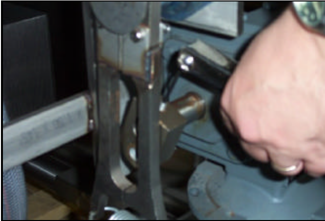
Loosening the set screw with the 1/8 allen wrench.
