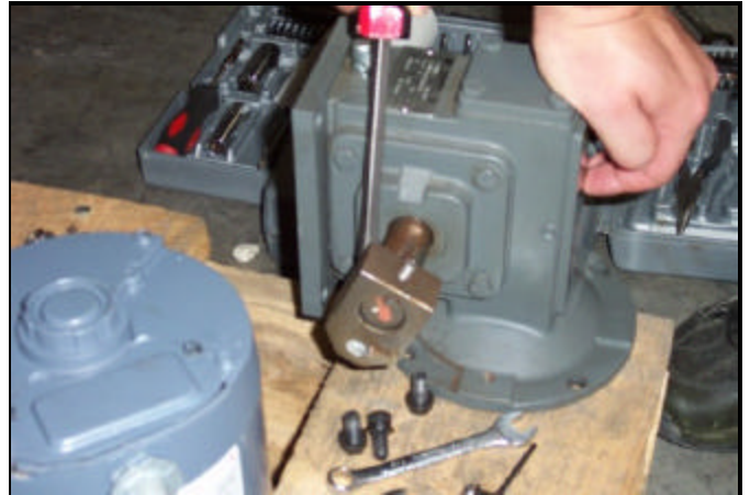
Removing the drive hub.
