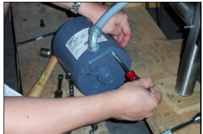
Removing the wiring access cover.
