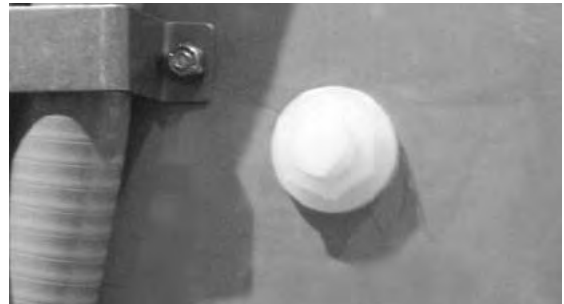
Detergent Connection Point (Machine rear view)
