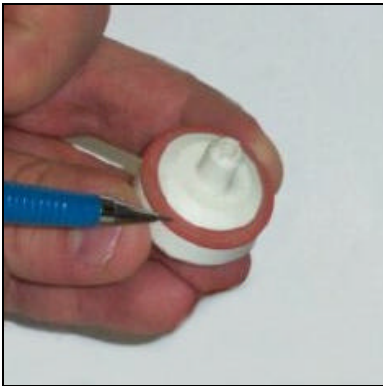
Examining the seal ring on the plunger
