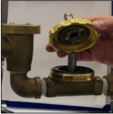
Removing the valve bonnet
