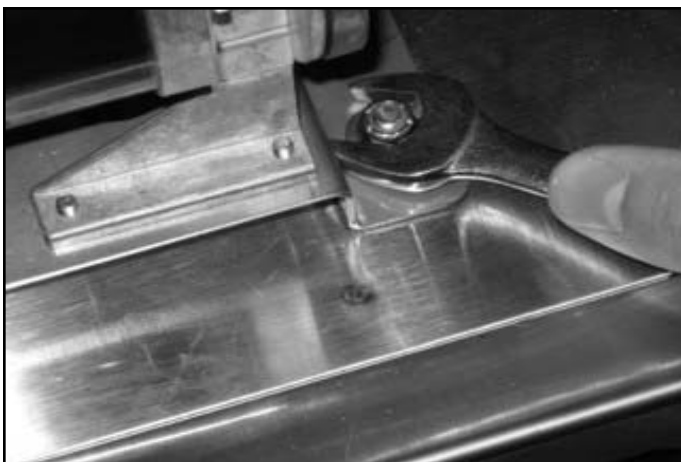
Removing the assembly mounting nuts.
