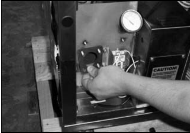
Removing the heater gasket
