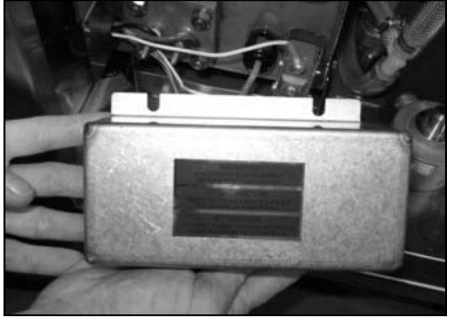
Removing the heater cover.
