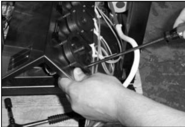
Removing the motor mounting screws.
