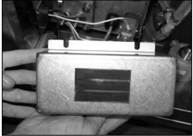
Removing the heater cover.
