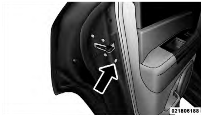
Child-Protection Door Lock Location
