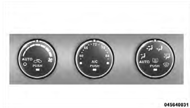
Automatic Temperature Control
