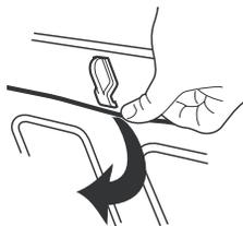
2. Lower the front of the broil element to access the ceiling for cleaning.
