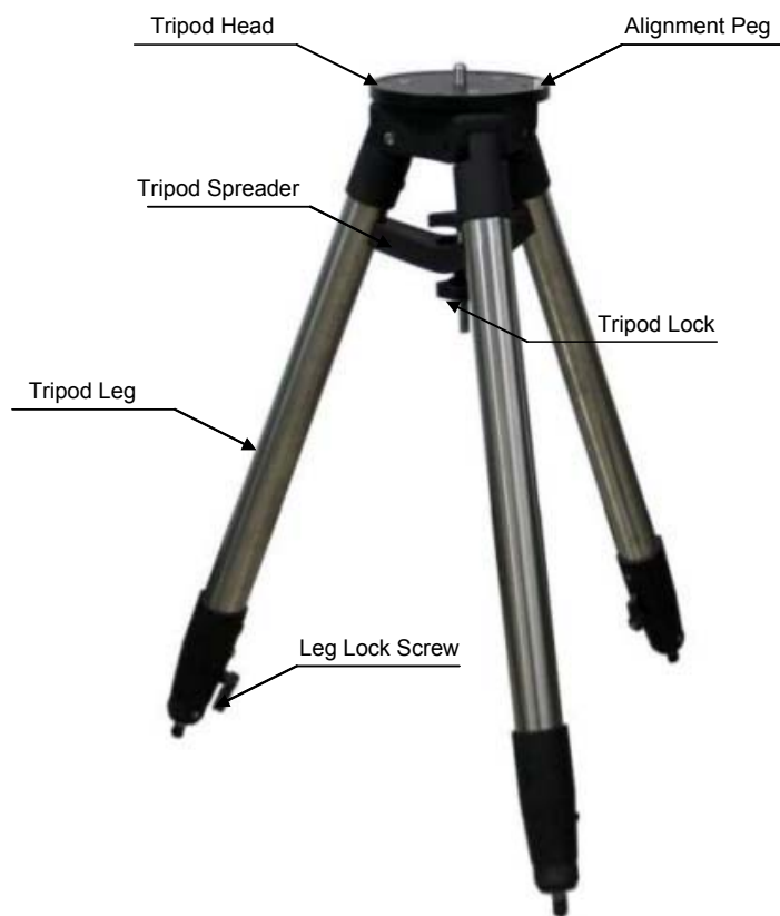
Figure 5. iEQ75-GT assembly terms (mount and optional tripod)
