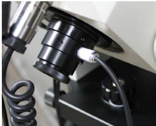
Figure 12. Connect the illumination LED to Polar Scope
