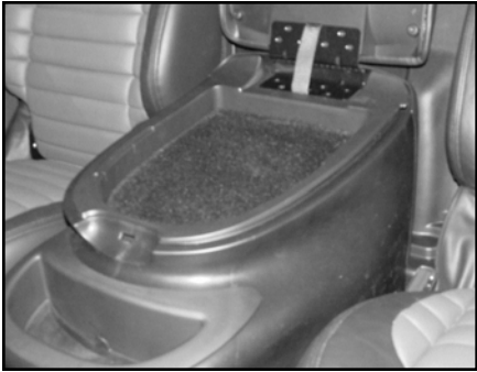
STEP 23: Replace front pocket that was removed in STEP 1 and close the lid.
