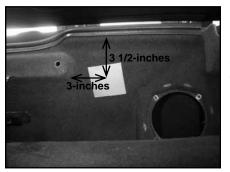
**STEP 5** Place a supplied wax squares onto the driver's side of the rear bulkhead.
