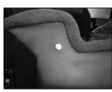
**STEP 6** Fully thread in each supplied 3/8-inch hex head bolt into each Stealthbox<sup>\*</sup>.
