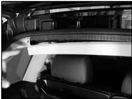
STEP 6 Remove the top sill plate.
