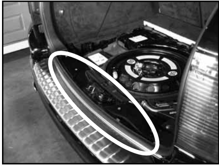
STEP 4 Remove the bottom sill plate.
