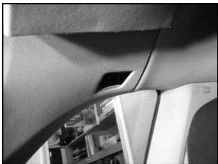
STEP 7 Remove the plastic cover from the upper d-pillar trim. Remove the phillip head screw that has been exposed .
