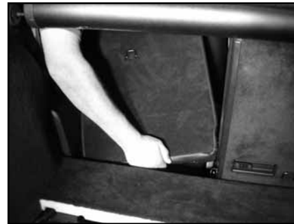
STEP 10 Grab a hold of the back of the driver's side rear seat as in the picture. Lift the right side of the seat up and out of the hinge bracket. Pull the left side of the seat towards the middle of the vehicle, sliding the seat off of a hinge pin. Once the seat is off both hinge points, remove the seat from the vehicle.
