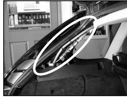
STEP 8 Remove the upper d-pillar trim.
