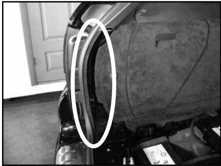
STEP 5 Remove the lower d-pillar trim.
