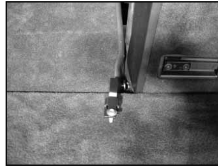
STEP 9 With a T-30 socket, remove the bolt and metal bracket that is located between the two rear seats.
