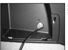
Run speaker wire from the amplifier location to the Stealthbox® location.
