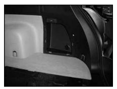
Remove the passenger's side rear pocket door and the separation wall.
