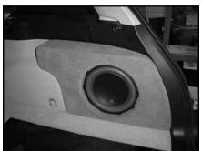
STEP 8 Position the Stealthbox® in the mounting location and press on it firmly.
