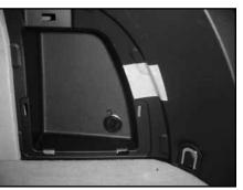
STEP 6 Apply the supplied wax square into place. The left side is lined up with the left edge of the pocket opening and above the emboss portion of the inner lower corner.
