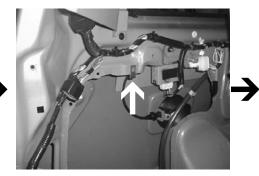
**STEP 12:** Insert the supplied U-bolt in factory hole.
