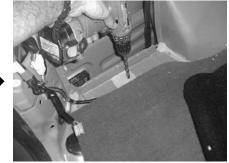
**STEP 10:** Using a 1/2" drill bit, drill a hole through the metal floor in the location of the impression in the wax square.
