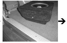
**STEP 7:** Insert supplied Socket Set Cup Screw into the enclosure so the rod extends approximately 1/4" out of the enclosure.
