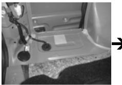
**STEP 8:** Roll the floor carpet back to expose the metal floor in the location shown above. Place the supplied wax square on the metal floor as shown above.
