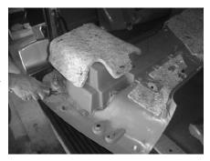
**STEP 3:** Grind off the plastic tabs which hold the pocket to the panel.
