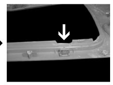
**STEP 6:** Create a second notch in the side panel as shown in the picture.
