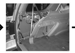
STEP 2: Remove the driver's side rear panel.
