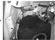
**STEP I5:** Place the Stealthbox in its proper location, making sure to place the threaded rod into the previously drilled hole in the floor.
