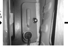
**STEP 15:** Adjusting the Socket Set Cup Screw so that the proper length is exposed (the exposed end of the rod is slotted to accept a flat-blade screw driver to be used when adjusting the rod's position). Place the 3/8" flat washer, 3/8" lock washer and 3/8"bolt, in that order, on the threaded rod. Do not fully tighten.
