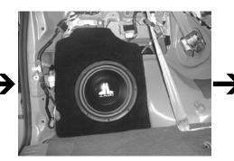
**STEP 17:** Fully tighten the bolt on the top of the enclosure and the nut on the threaded rod on the bottom of the enclosure to secure the enclosure.
