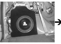
**STEP 9:** Place the Stealthbox into place so as to allow the Socket Set Cup Screw to make an impression in the wax square.
