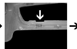
**STEP 5:** Create a notch in the side panel as shown in the picture.
