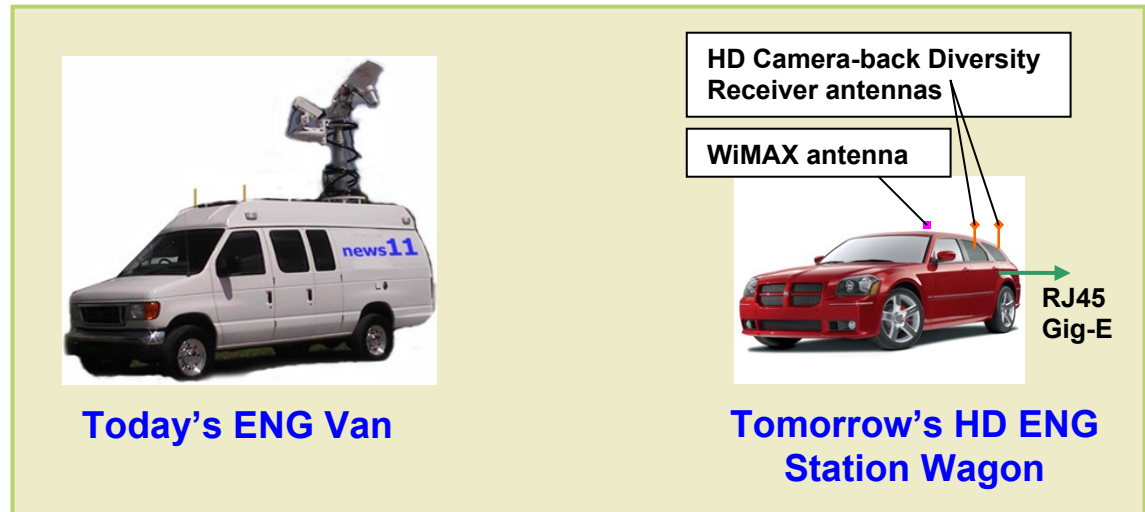
Fig. 15. In less than 5 years, HD ENG backhaul may be accomplished through a combination of WiMAX and Fiber IP within a metropolitan area. Frequent ENG program origination points may have pre-wired Fiber IP network connections while other points are in proximity to WiMAX service. The traditional large ENG Van, with costly microwave electronics, dish antennas and telescopic masts, may only be used for rural reporting where WiMAX and Fiber IP are not available.
